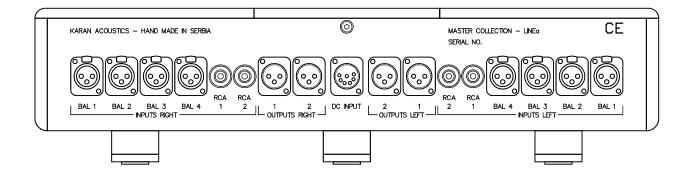
On the main control unit rear panel there are *four (4) XLR* and *two (2) RCA* line inputs, *two (2) XLR* main outputs and *one (1) 7-pin XLR DC voltage input*.
