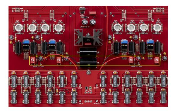
Inside the Main Control Unit chassis there are arrays of DIP switches *(4 in total, marked SW-1 on the motherboard top side)* and can be clearly seen on this image.
