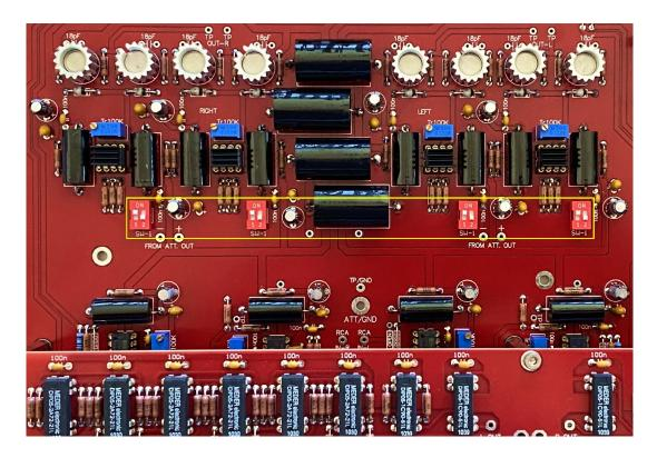
Inside the Main Control Unit chassis there are arrays of DIP switches *(4 in total, marked SW-1 on the motherboard top side)* and can be clearly seen on this image.
