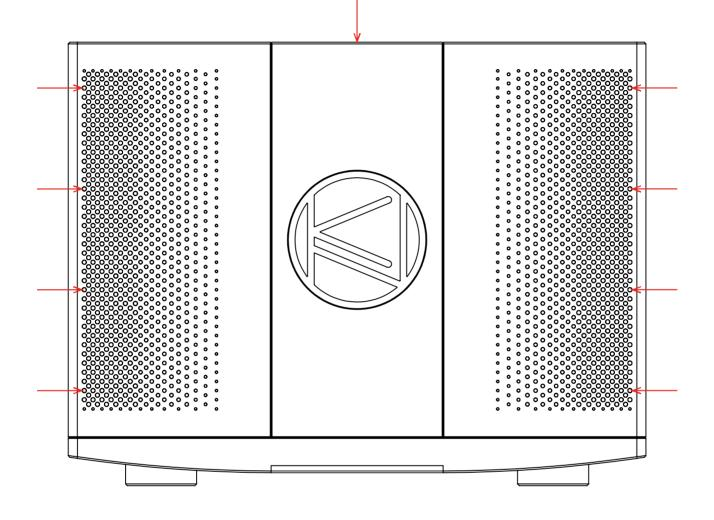
Top cover is fixed to the main chassis by *eight (8) hidden allen screws*. Locate *eight (8)* clearly marked positions with acces holes in the top cover. Using the supplied *allen key No.3* reach each screw carefully through the holes in the top cover and release the screws. Using the same allen key release *one (1) remaining*, clearly marked screw in the centre *(middle)* of the back panel.
